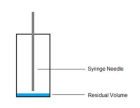
Unlike other vials, the  $AQ^{\text{TM}}$  and  $RSA^{\text{TM}}$  brand Vials have a specification for bottom height. This specific tolerance of the bottom height allows you to bring the needle down to the lowest position necessary.
